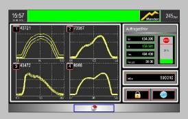
The **Mandonic** auto enveloping system adjusts the envelope limits according to the current variation of the process.
