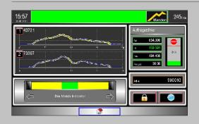
The **DMI** Die Match Indicator assists operators in aligning thread roll dies quicker, more precisely, and more efficiently, and it extends tool life and improves thread quality.
