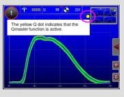
SKQmaster stabilizes the horizontal offset. It is now possible to operate the system with a much more narrow envelope limit range. The number of unnecessary machine stops is reduced.
