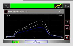
The optional **SK**Partmaster shows the operator the target force curves which can be viewed while the machine is running. A direct comparison is shown between the memorized good target curve (grey band) and the current force signal (white). Set-up problems are identified immediately and can be corrected to bring the process back into the desired operating range.
