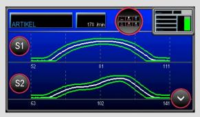
Dynamic envelope monitoring is applied to all channels. Up to (2) channels can be monitored.
