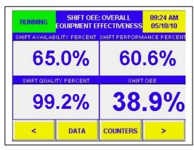
This screen displays the **SHIFT OEE** values for the machine. The Shift OEE is calculated by multiplying the Availability Percent, the Performance Percent, and the Quality Percent. These real-time values are continuously available to operators and managers on the shop floor as well as to other management staff through TSS-NET.
