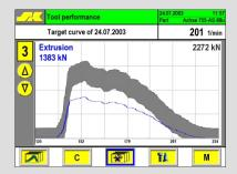
The optional **SK**Partmaster shows the operator the target force curves which can be viewed while the machine is running. A direct comparison is shown between the memorized good target curve (grey band) and the current force signal (blue). Set-up problems are identified immediately and can be corrected to bring the process back into the desired operating range.
