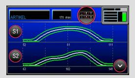
Dynamic envelope monitoring is applied to all channels. Up to 8 channels can be monitored.
