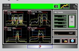
The main screen shows the signals of all connected sensors and the memorized envelope curves.
