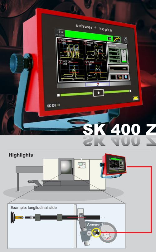
Easy to install sensors are bolted onto machine parts which are taking the loads from the cutting process such as drive arms for longitudinal or cross slides. These sensors measure the cutting forces and/or the acoustic emission signals. Alternatively, electrical power sensors are registering the power consumption of the electrical drive motors.
