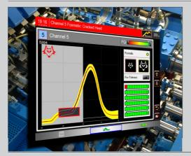
Foxmatic uses the latest pattern recognition procedures to detect random faults such as cracked heads. Based on its new drift compensation technique, Foxmatic recognizes the "fingerprint" of the error and can tell the difference between errors and normal process variation. Foxmatic reacts to even the smallest chages in the force signals and stops the machine. The error display offers a review of the last sixty (60) forming cycles.
